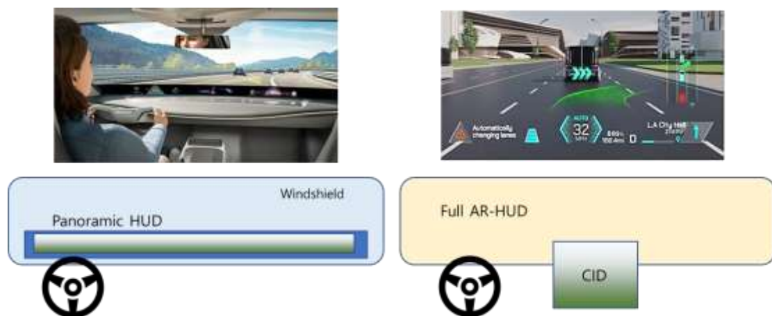
Fig. 1. Future vehicle display example based on HUD technology
