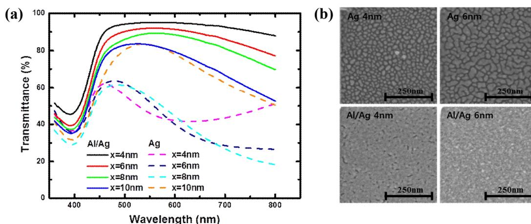
**Fig. 1. (a) Optical transmittance spectra of the Glass/Alq3(60nm)/LiF(1nm)/Al(1nm)/Ag(x)/Alq3(60nm) (solid line) and Glass/Alq3(60nm)/LiF(1nm)/Ag(x)/Alq3(60nm) (dotted line) as the thickness of the Ag layer. (b) SEM images of the Ag and Al/Ag surfaces at the sample with the Ag thickness of 4, 6nm.**
