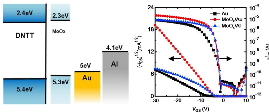
Fig. 1. Energy band diagrams and transfer characteristics of the DNTT-based TFTs with various contact metals in a linear regime where  $V_{DS} = -3V$ .
