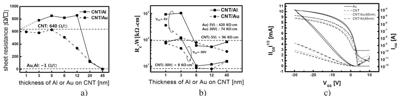
Figure 1 a) The sheet resistance and b) the contact resistance of CNT/metal hybrid electrodes according to thickness of Au and Al layer on CNT, c) the transfer curves of pentacene OTFTs using the CNT/metal hybrid electrodes.
